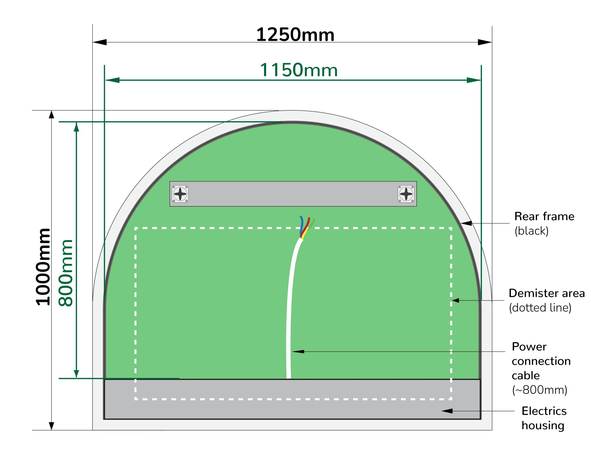
When connecting your mirror to the mains lighting circuit, the green area shown above represents the safe zone for you to drill and connect to your power cable. There is not a small, exact cable entry that you have to align with - and this gives you greater flexibilty when it comes to fitting/connecting your mirror to the mains.
