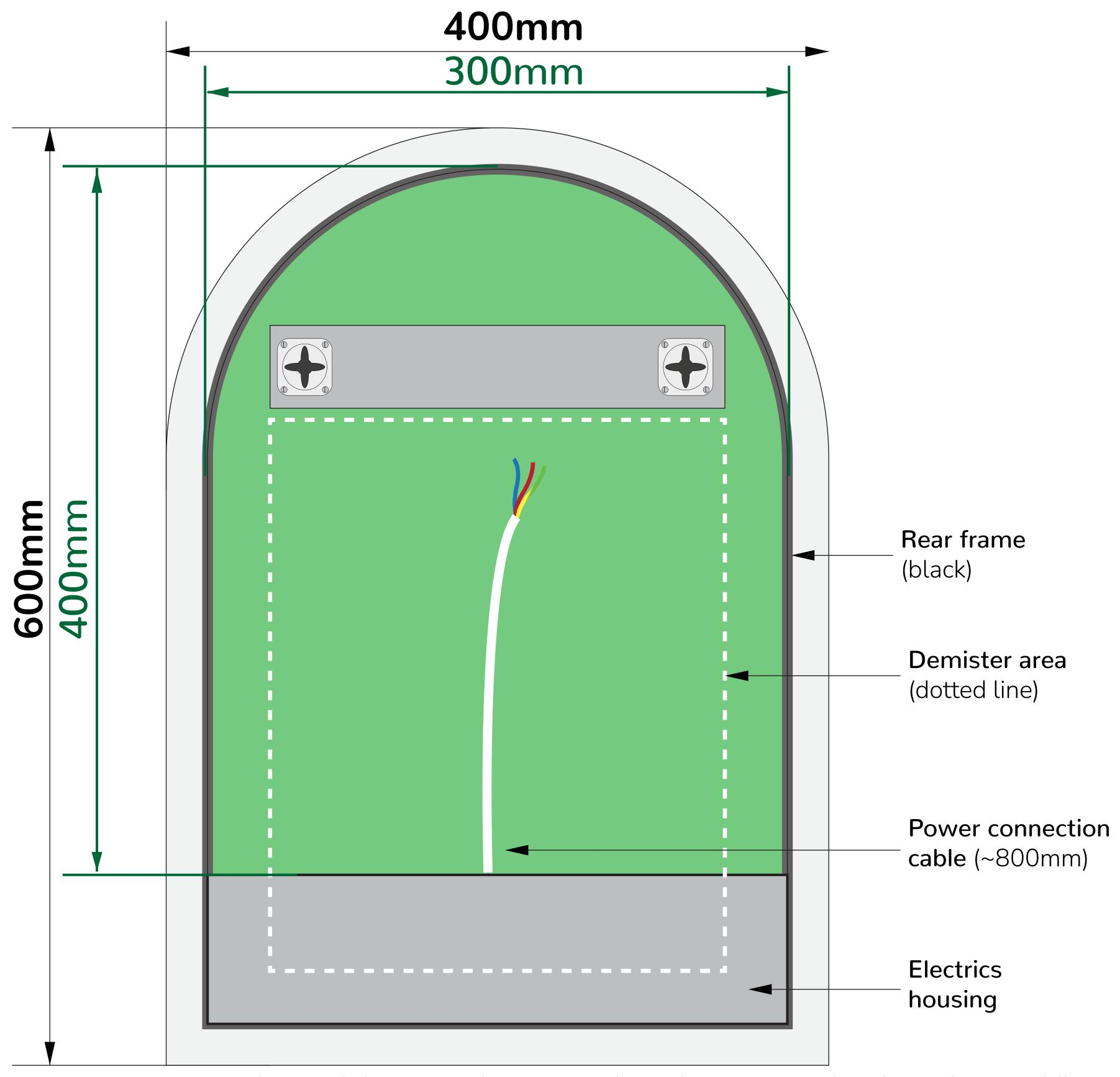
When connecting your mirror to the mains lighting circuit, the green area shown above represents the safe zone for you to drill and connect to your power cable. There is not a small, exact cable entry that you have to align with - and this gives you greater flexibilty when it comes to fitting/connecting your mirror to the mains.
